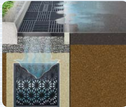
Flo-Grid® porous paving for edge drainage and infiltration.
